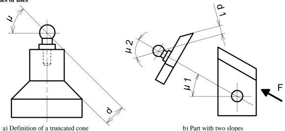
These two simple examples show how tooling balls are used. In order to tool or control part b) in the usual way, two tooling holes would be necessary, one of them oblique, which would bring problems and added up inaccuracies.
